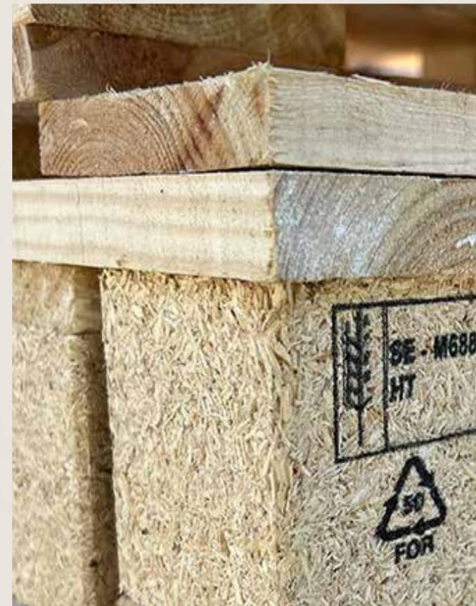
At their state-of-the-art facility, returned and end-of-life wooden pallets are ground into wood chips, which are then mixed with a small amount of glue and pressed into high-quality chip blocks. These blocks are directly reintegrated into new pallet production, extending the life cycle of materials and reducing waste.
